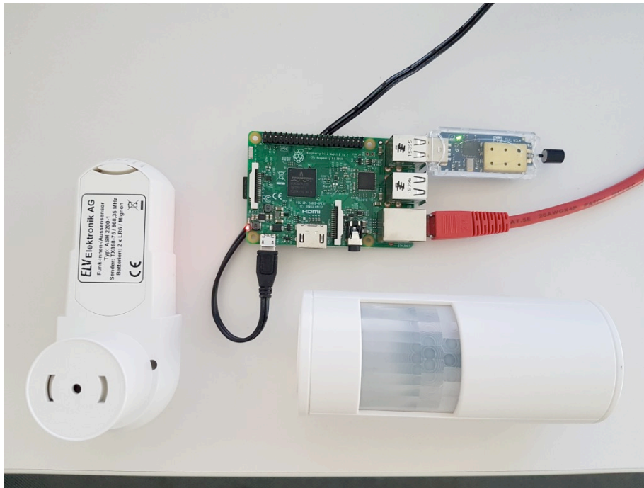
Figure 5: OpenMTC gateway on Raspberry Pi with attached sensors
